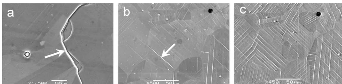
Fig. 7. Morphologies of slip channels on the surface of irradiated samples strained in argon at 288 °C: (a) 15Cr12Ni at 5 dpa and 1%, (b) 21Cr32Ni at 1 dpa and 1% and (c) 21Cr32Ni at 1 dpa and 3%.
